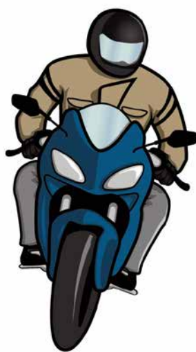
Front wheel momentarily out-tracks away from turn, causing motorcycle to begin leaning in turn direction.
